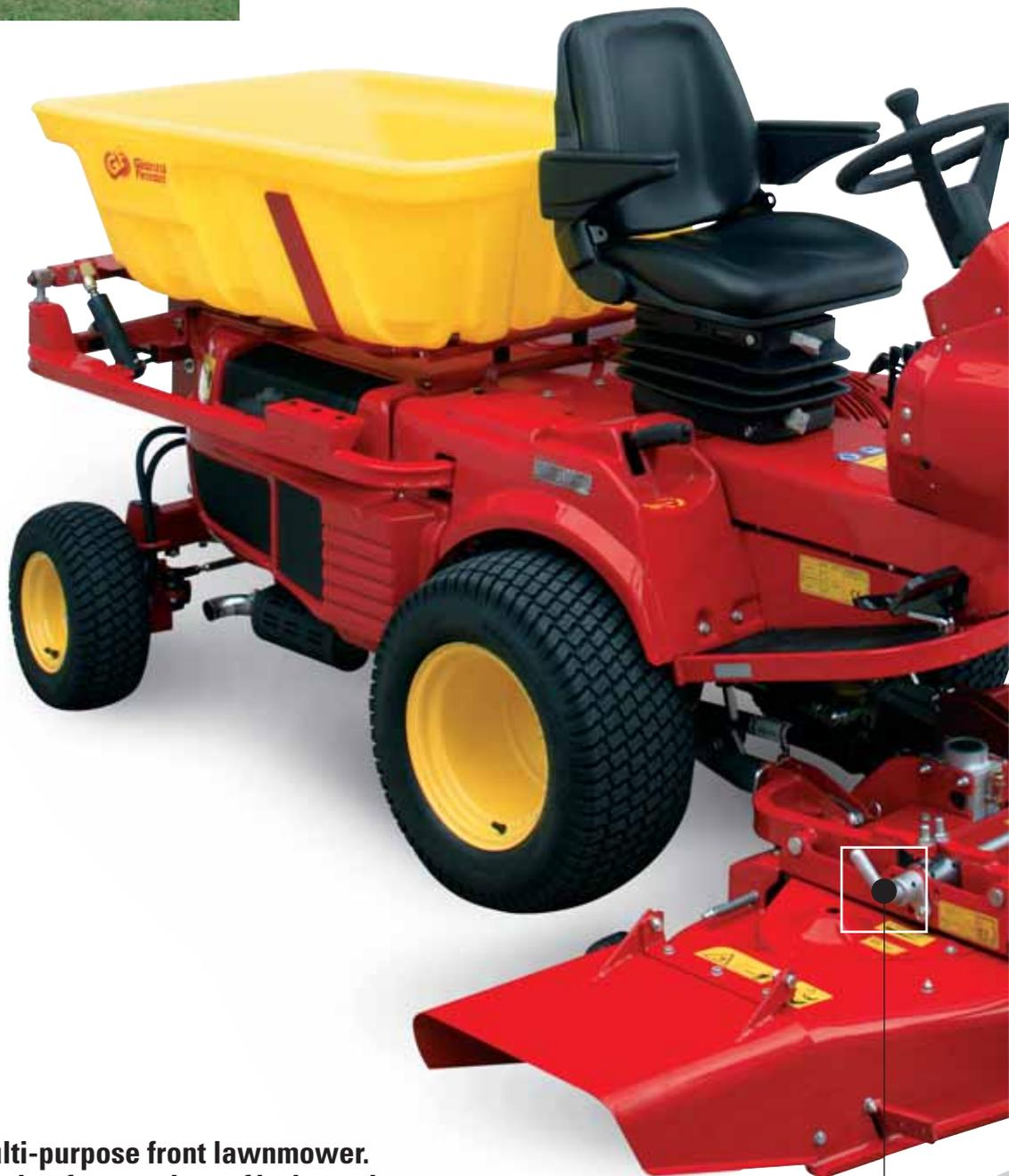
**SR machines** are multi-purpose front lawnmower. The SR product family includes four versions of hydrostatic machines with petrol or diesel engines and 2 or 4 wheel drive. With SR lawnmowers several attachments can be fitted to ensure an increased return on investment for landscapers and other professionals.
